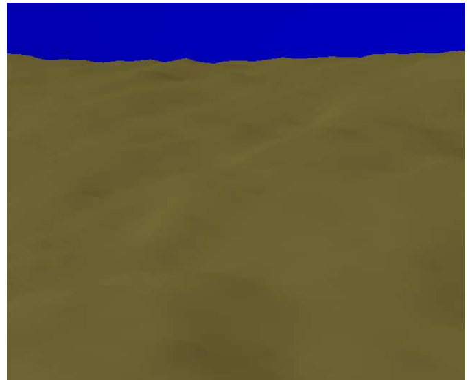
Figure 75: The ground a muddy color under water. The light is also made more ambient to simulate the scattering effect of the water and particles therein
