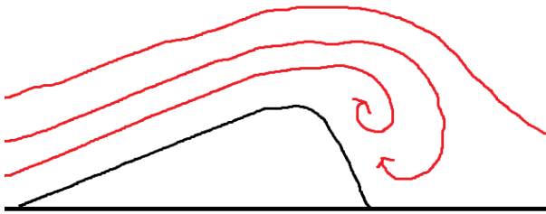
Figure 77: Wind blows particles up the leading edge of the drift and then swirls around over the top. This results in a steeper leeward side with particles in effect being blown into the drift against the general wind direction.
