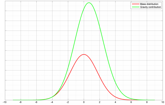
Figure 9: It is seen that the mass closest to the detector, at the right hand side, contributes more to the gravitational pull than the mass to the left.
